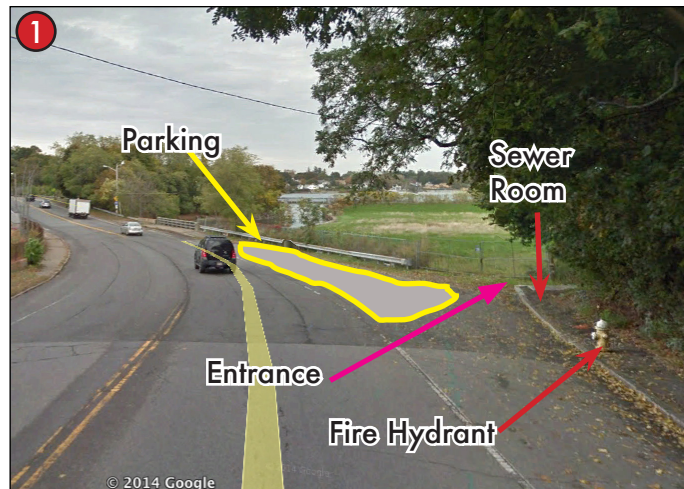
The small parking bump-out is restricted by an underground sewer room and fire hydrant that need to remain accessible.
