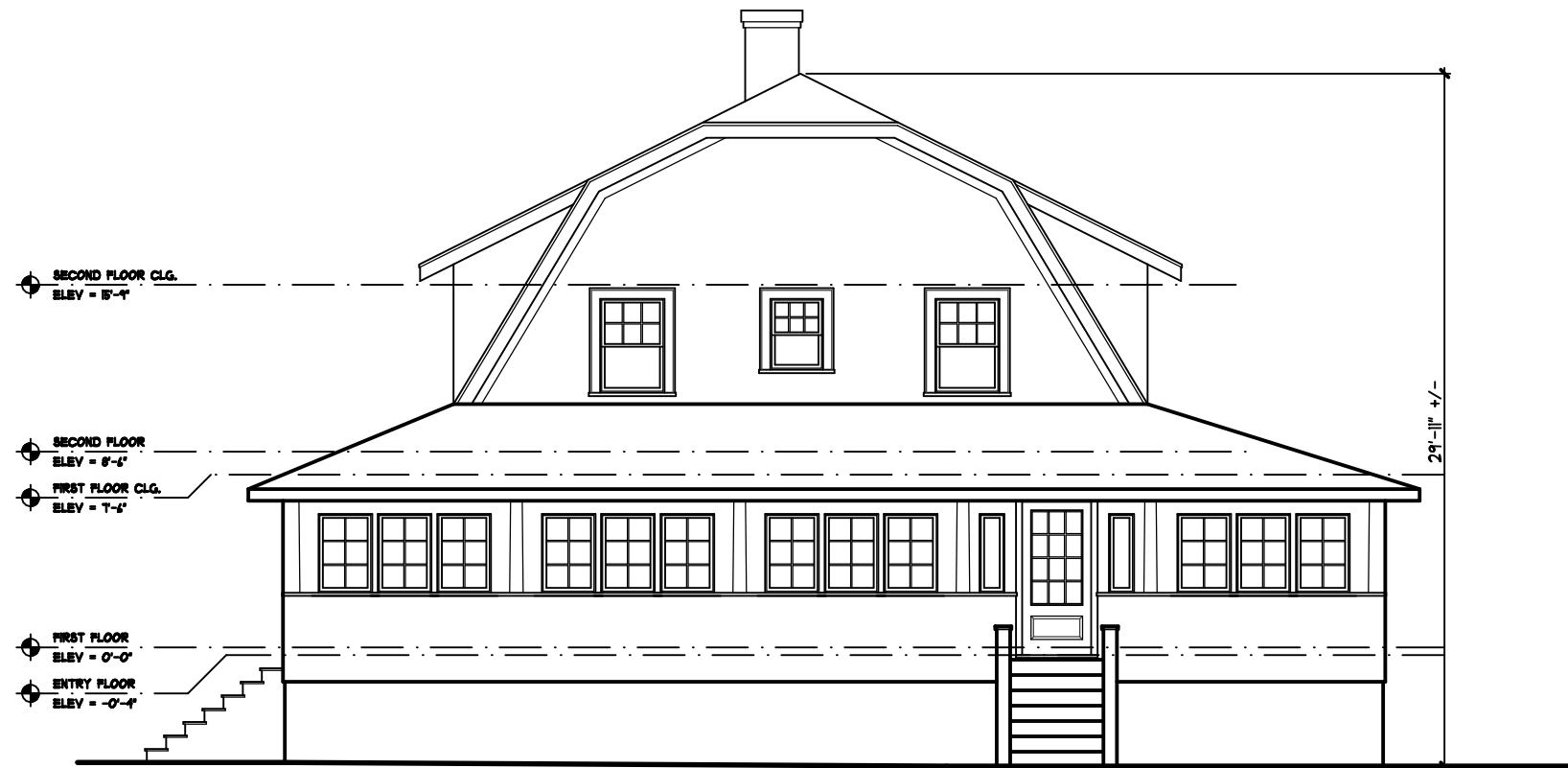
1 EXISTING FRONT ELEVATION
