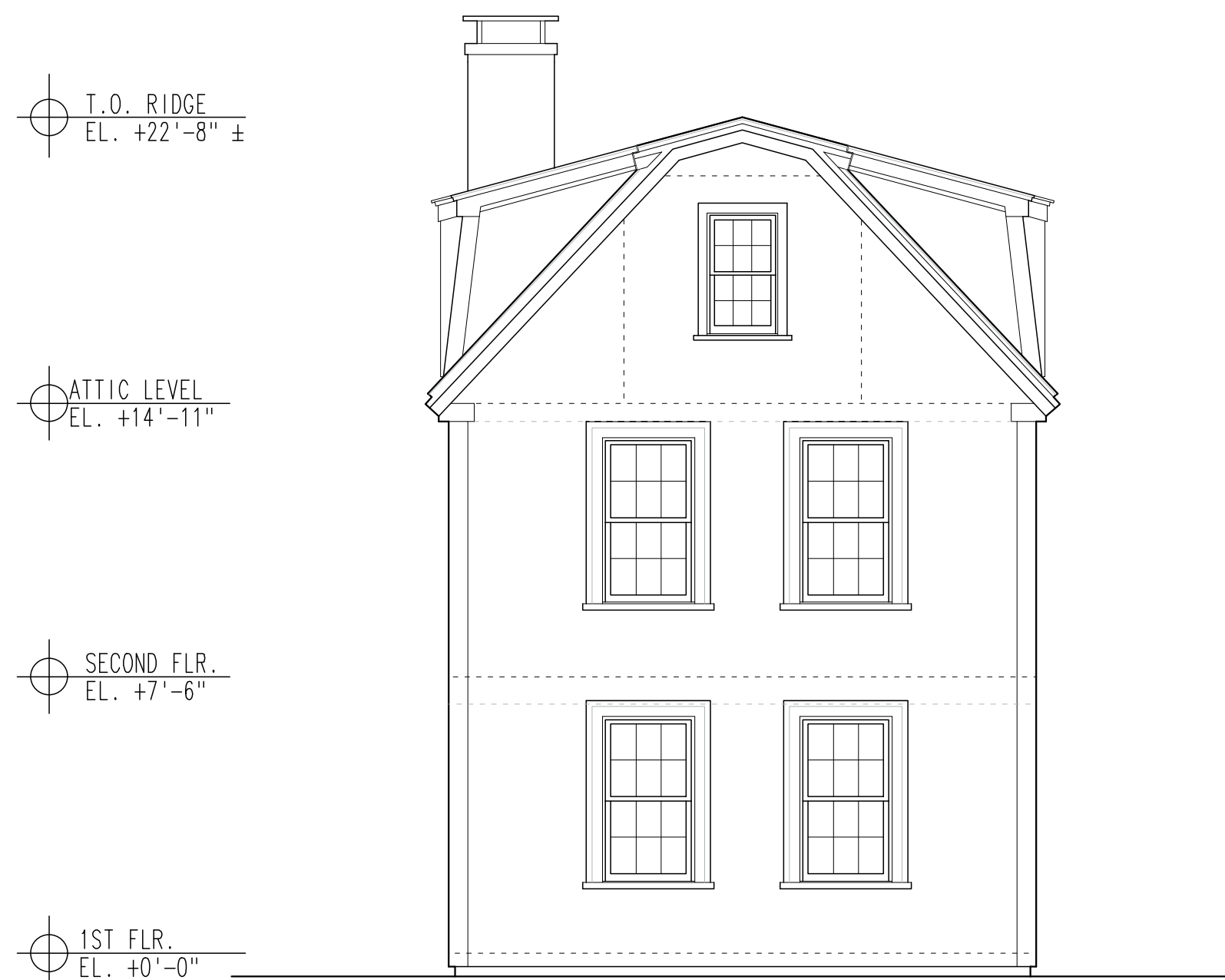
1 EXISTING/NEW FRONT ELEVATION- SOUTH 3/26/21
