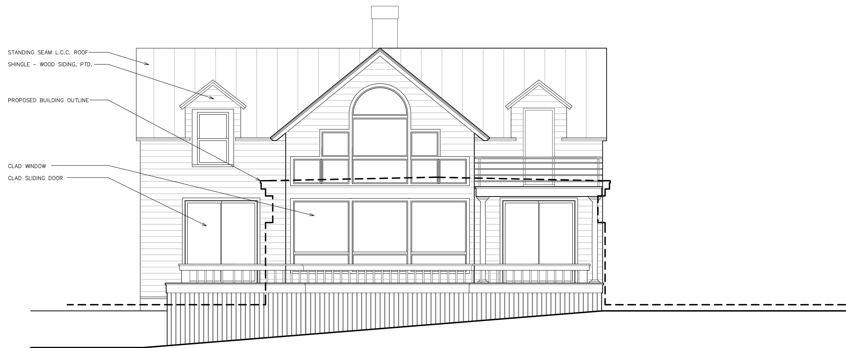
2 EXISTING EAST ELEVATION - 5 GILBERT HEIGHTS RD 1/4" = 1'-0"
