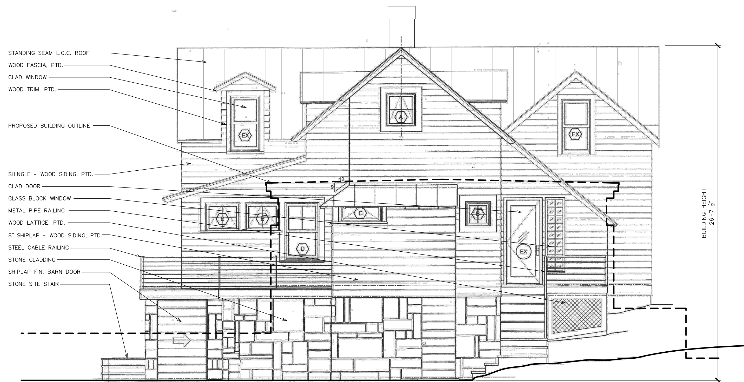
4 EXISTING WEST ELEVATION - 5 GILBERT HEIGHTS RD 1/4" = 1'-0"
