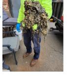
moved from the Green Street Pumping Station. This blockage prevented the sewer from flowing properly and resulted in the backup.
