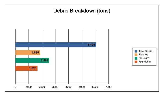
The model estimates that a total of 6,100 tons of debris will be generated. Of the total amount, Finishes comprises 31% of the total, Structure comprises 42% of the total, and Foundation comprises 27%. If the debris tonnage is converted into an estimated number of truckloads, it will require 245 truckloads (@25 tons/truck) to remove the debris generated by the flood.
