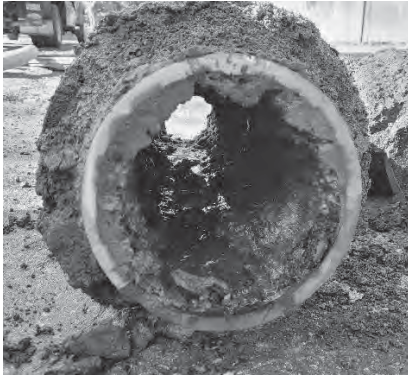
Figure 1 – Buildup of tuberculation on the interior of the Humphrey Street pipe prior to cleaning and lining
